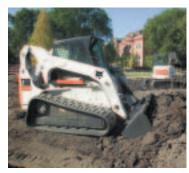
After a heavy rain, tracks get you back on the job sooner. A solid-mounted track undercarriage provides consistent tractive effort for extra pushing power and smoother leveling.
